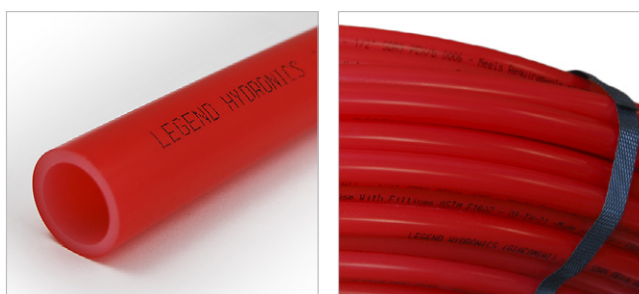
The externally-extruded EVOH oxygen barrier reduces oxygen molecule permeation into the water. Compliant with standard DIN4726 (<0.1 grams/m 3 /day).
